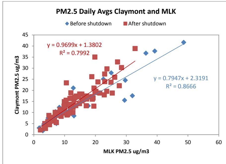
The correlation between PM2.5 at Claymont and MLK did not show any significant difference before and after the Evraz shutdown. PM2.5 concentrations at both sites were well correlated.
