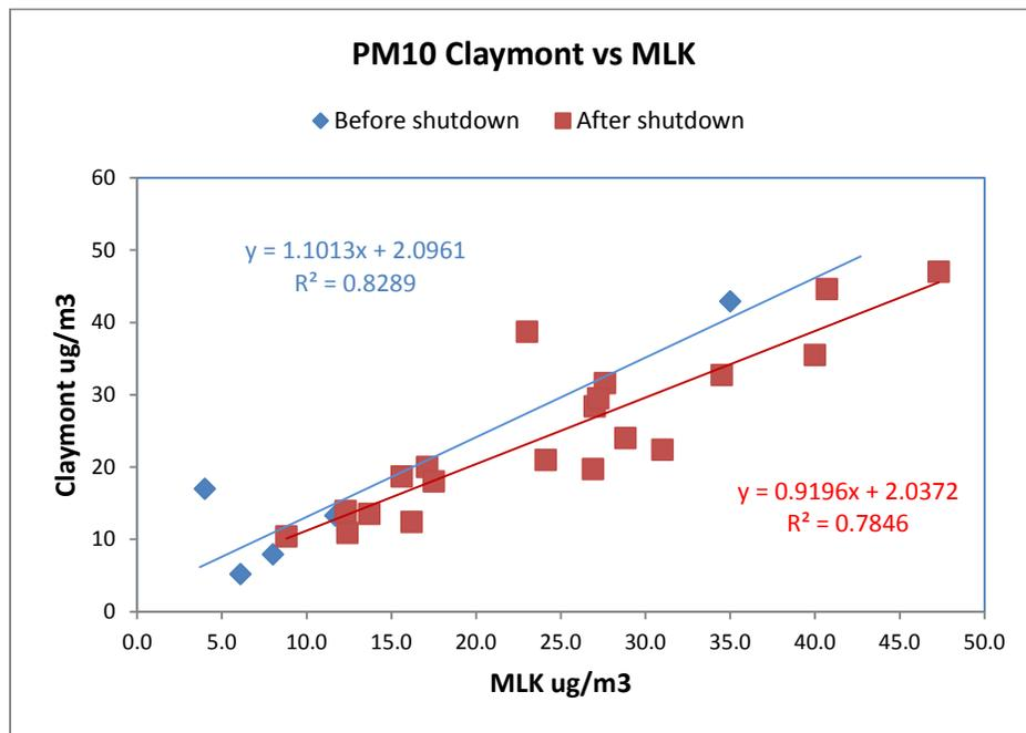
Comparing the time series and the correlations for the PM10 concentrations at Claymont and MLK both before and after the Evraz shutdown does not show any significant difference at Claymont relating to the shutdown.
