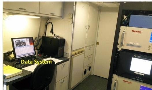
A Data Acquisition System used in the Delaware ambient monitoring network was installed for real-time retrieval of 1 minute, 5 minute, and hourly average data from the continuous monitors. A wireless internet connection allows remote access to data and the security cameras mounted outside the vehicle.
