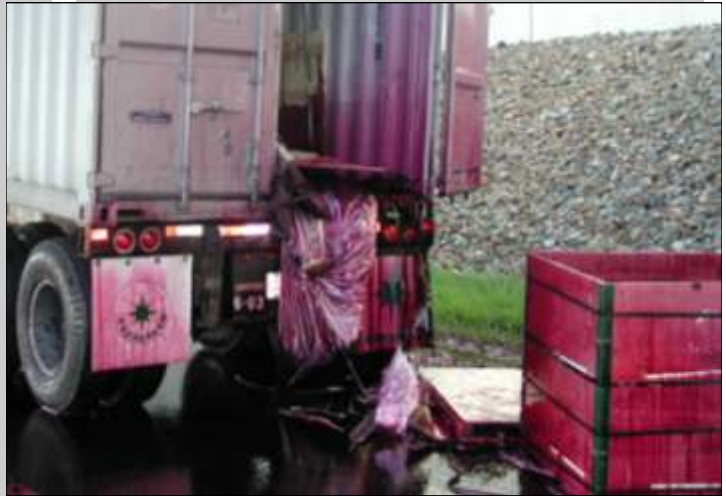
A broken tote and ruptured liner are strewn about at the scene of the grape juice incident.
