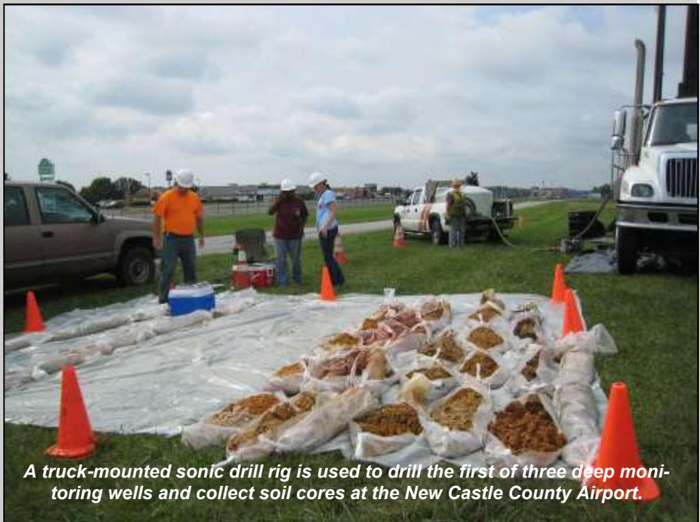
*A truck-mounted sonic drill rig is used to drill the first of three deep monitoring wells and collect soil cores at the New Castle County Airport.*
