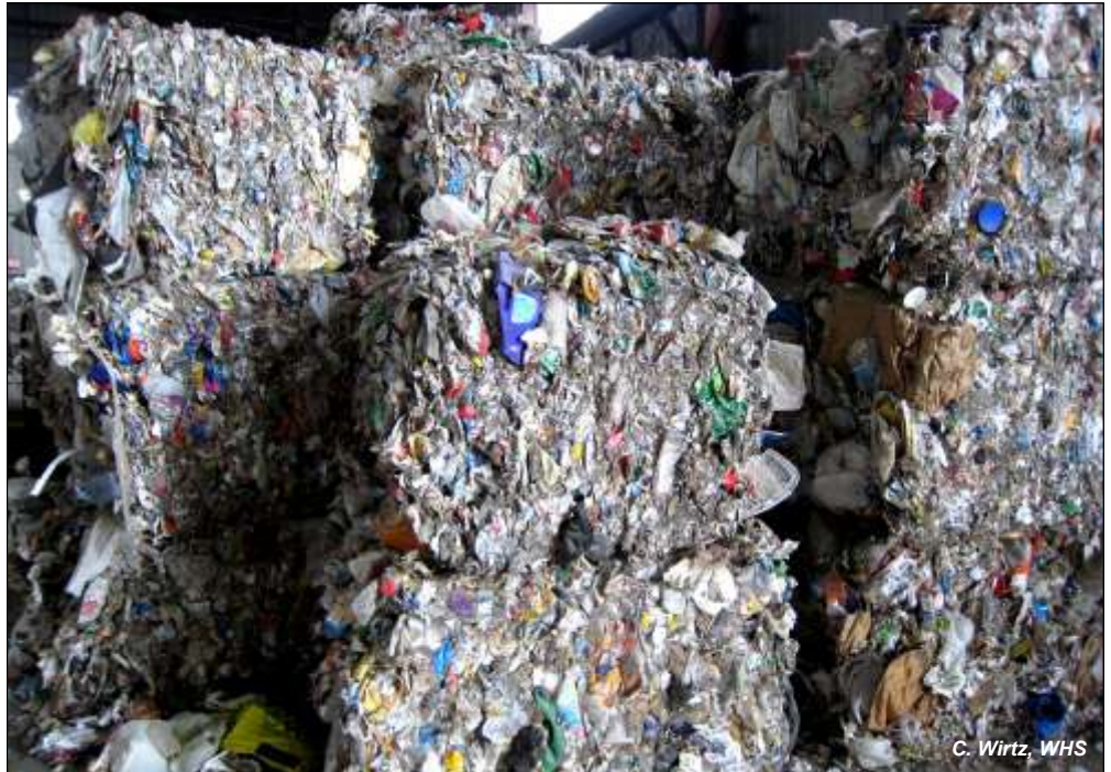
Baled household plastics at the new Blue River Resources materials recovery facility in Wilmington. Each bale weighs close to one ton.
