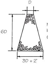
NOTE: Stabilized outlet to be underlain with GS-1 geotextile
