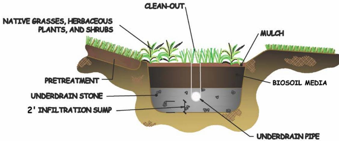
Figure 2.1. Traditional Bioretention Underdrain Design
