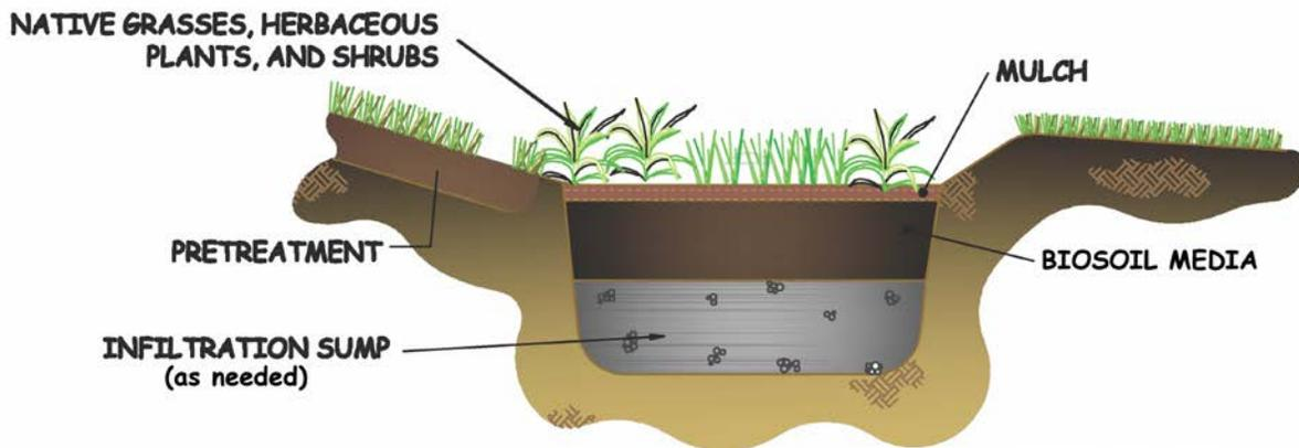
Figure 2.2. Traditional Bioretention Infiltration Design
