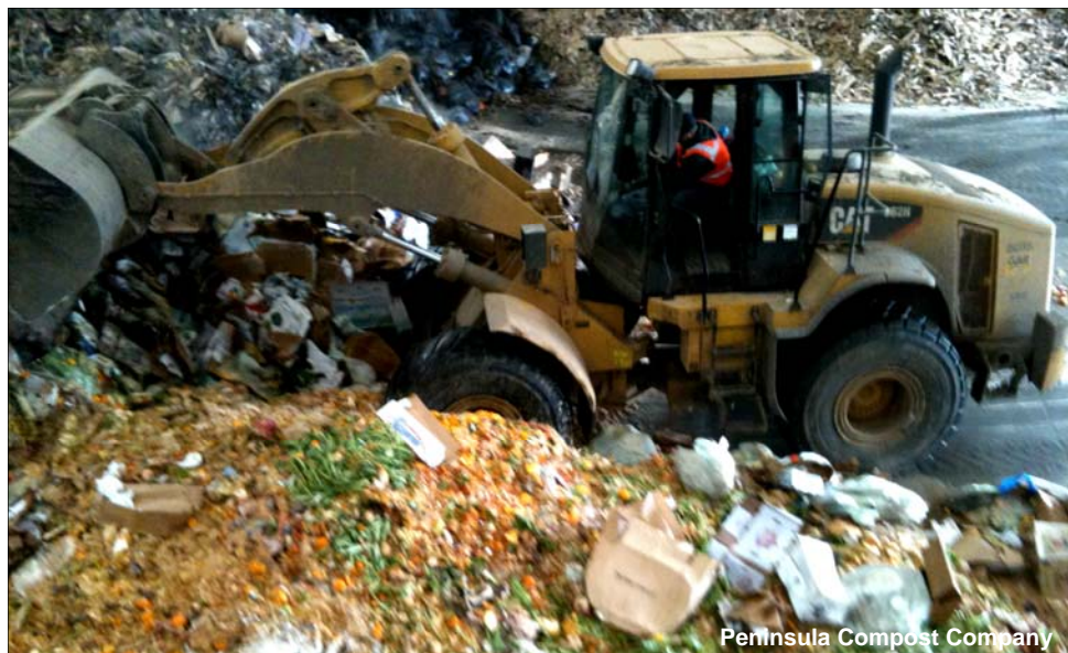
A front-end loader is used to stage the food waste inside the warehouse.
